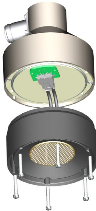
FIGURE 9. Remove Transducer Housing and Disconnect Wires
